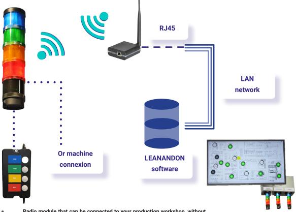
Radio module that can be connected to your production workshop, without being connected to a PC.
