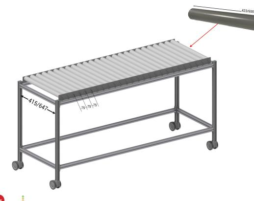
Conveyor rollers are intended to ensure the transfer of boxes or products.
